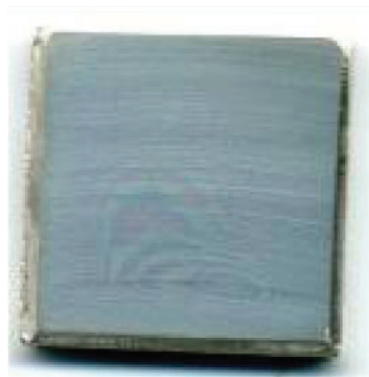
10 Picture of sample surface after exposure to O_2+N_2+RH+UV for 22 h. Specific conditions: flow-rates of 89.2\text{ cm}^3\text{ min}^{-1} O_2 , 803\text{ cm}^3\text{ min}^{-1} N_2 , 90% RH and UV radiation
