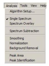
By default, a data processing/analysis method is applied to one spectrum at a time (note that *Single Spectrum* is checked by default). To set up a particular algorithm to use for each method, click *Algorithm Setup*.... The Analysis Setup window appears. Click on the page tab to bring up the algorithm setup page for a desired method.
