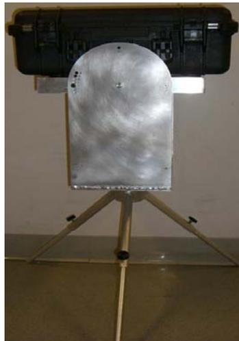
**Figure 4.1: Multi-Axis Differential Optical Absorption Spectrometer used in this research.**
