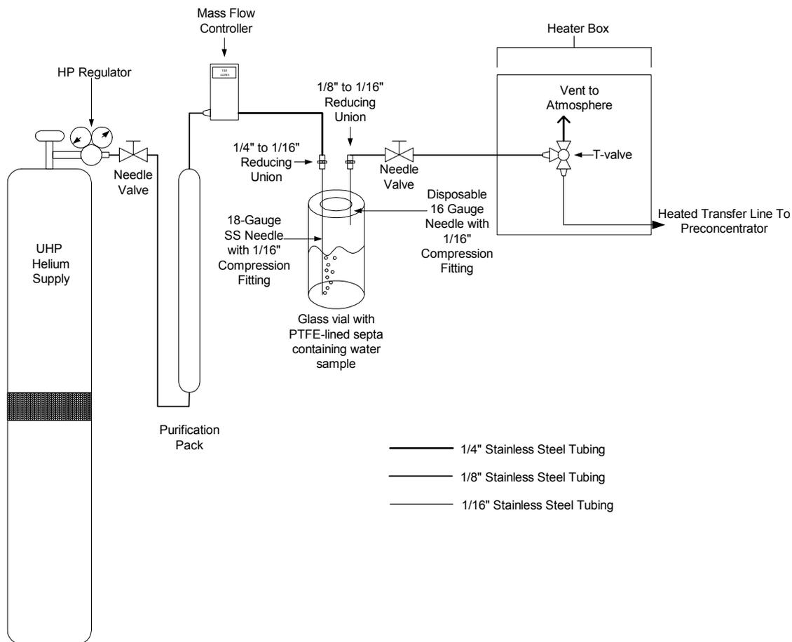
Figure 5.1: Detailed schematic of purge inlet system for water analysis. Components not to scale.
