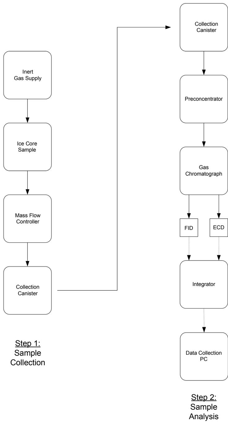
Figure 2.2: Block diagram illustration of ice core analysis experimental setup
