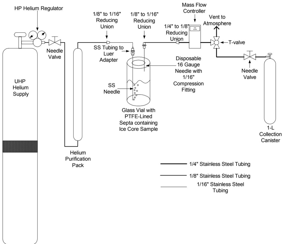
Figure 2.3: Detailed schematic of purge inlet system for ice core analysis. Components not to scale.
