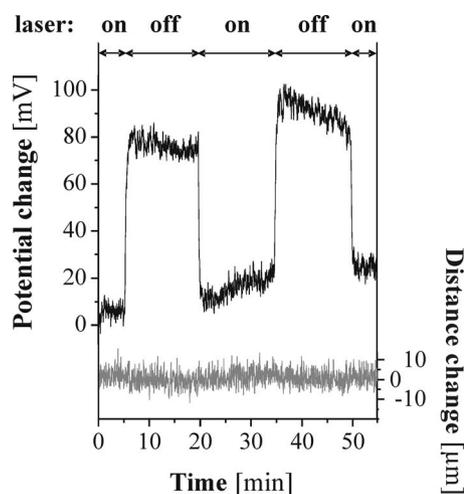
**Figure 3.** Potential and distance transients recorded on a ZnO-covered zinc foil irradiated with a 785 nm laser beam (output energy: 100 mW) focused beneath the KP needle.
