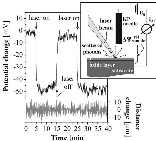
**Figure 1.** Potential and distance transients recorded on bare steel irradiated with a 785 nm laser beam (output energy: 100 mW) focused beneath the KP needle. Upper right corner: Schematic illustration of the experimental setup.<sup>1,2</sup>
