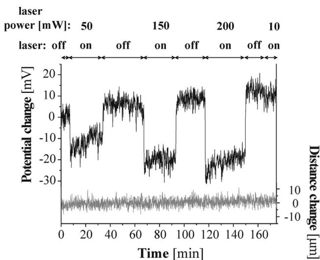
**Figure 2.** Potential and distance transients recorded on hematite-covered steel irradiated with a 785 nm laser beam focused beneath the KP needle and operated at output energies between 10 mW and 200 mW.
