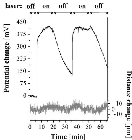
**Figure 4.** Potential and distance transients recorded on a Si wafer irradiated with a 785 nm laser beam (output energy: 100 mW) focused beneath the KP needle.
