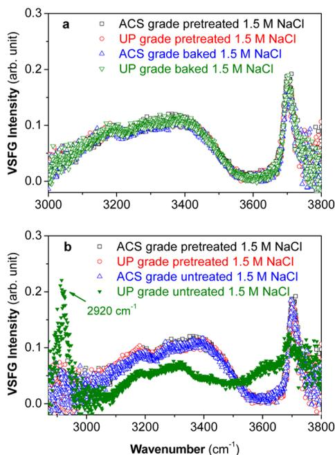
**Figure 4.** (a) Comparison between conventional VSGF spectra of baked or filtered 1.5 M NaCl solutions made from ACS and UP grade salts. (b) Comparison between conventional VSGF spectra of pretreated and untreated 1.5 M NaCl solutions made from ACS and UP grade salts.
