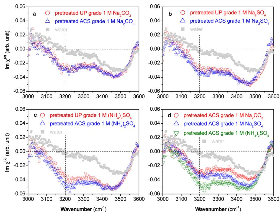
**Figure 2.** Comparison between HD-VSFG spectra from ACS and UP grade salt solutions after pretreatment. (a) 1 M  $\text{Na}_2\text{CO}_3$ , (b) 1 M  $\text{Na}_2\text{SO}_4$ , (c) 1 M  $(\text{NH}_4)_2\text{SO}_4$ , and (d) comparison of all 1 M salt solutions. The HD-VSFG spectrum of neat water is also shown as a reference.
