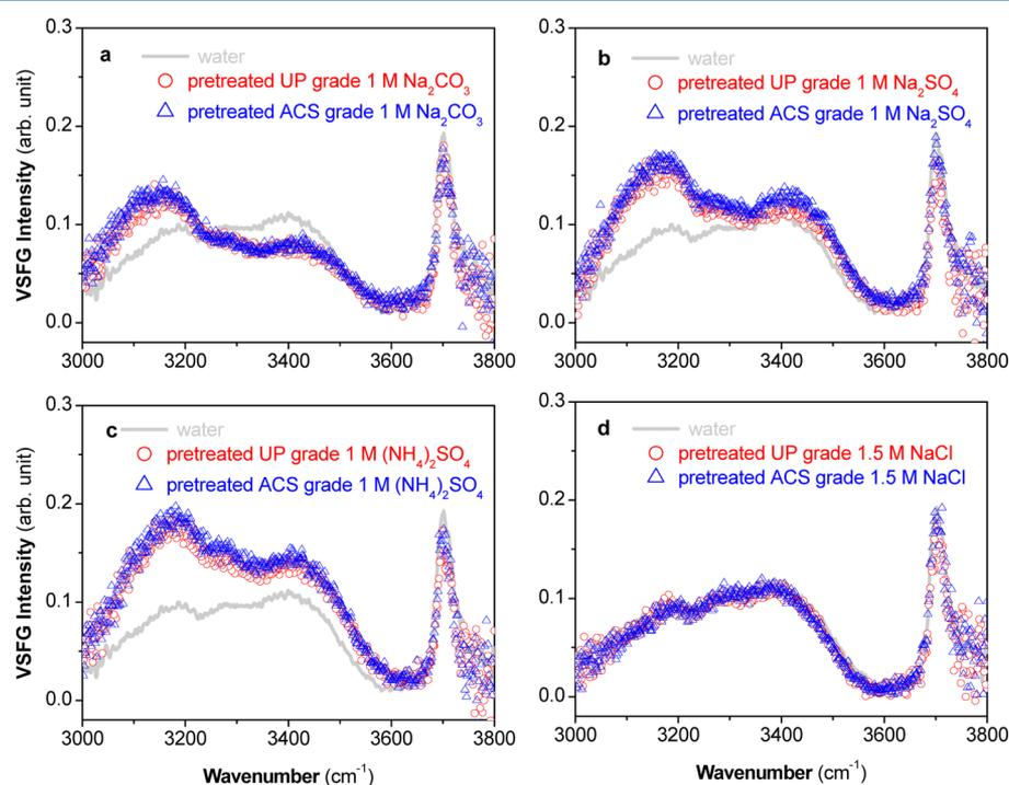
**Figure 1.** Comparison between conventional VSGF spectra from ACS and UP grade salt solutions in the OH stretching region (3000–3800  $\text{cm}^{-1}$ ) after pretreatment. (a) 1 M  $\text{Na}_2\text{CO}_3$ , (b) 1 M  $\text{Na}_2\text{SO}_4$ , (c) 1 M  $(\text{NH}_4)_2\text{SO}_4$ , and (d) 1.5 M NaCl. The VSGF spectrum of neat water is also shown as a reference by a gray line.
