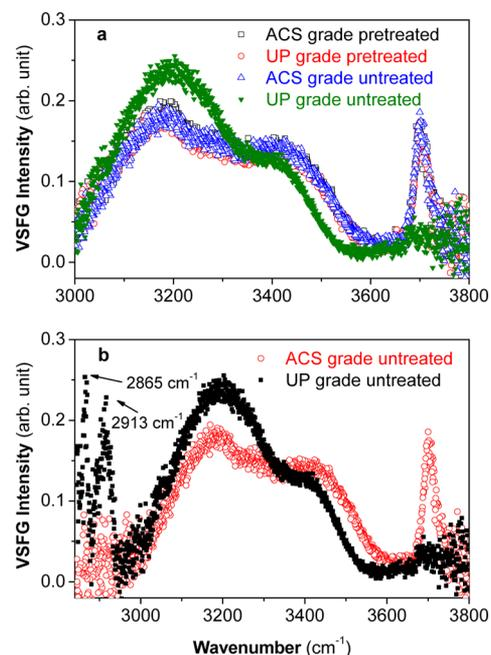
**Figure 3.** (a) Comparison between conventional VSGF spectra of untreated and pretreated 1 M  $(\text{NH}_4)_2\text{SO}_4$  solutions made from ACS and UP grade salts. (b) Comparison between conventional VSGF spectra of untreated 1 M  $(\text{NH}_4)_2\text{SO}_4$  solutions made from ACS and UP grade salts.
