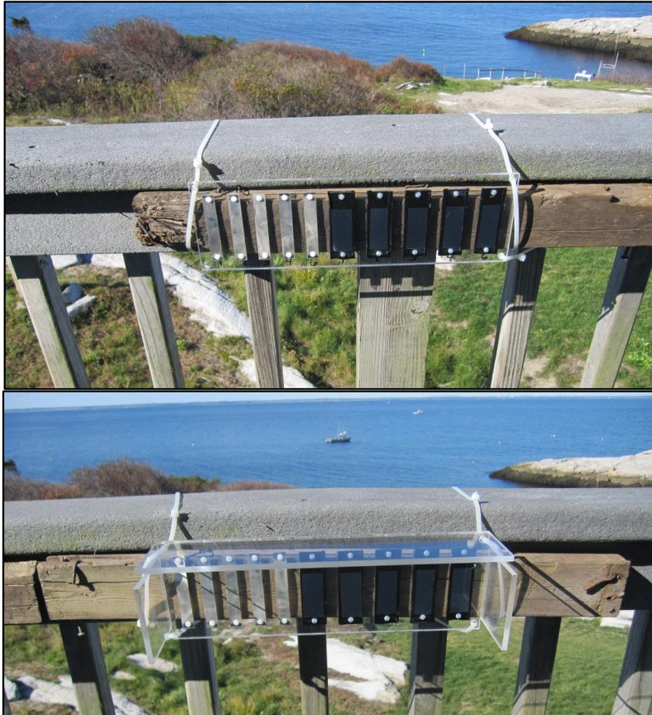
**Figure 2.2** Pictures showing the sample exposures at Appledore Island, ME. Top is unsheltered and bottom has a slight overhang to minimize contamination and wash-off.
