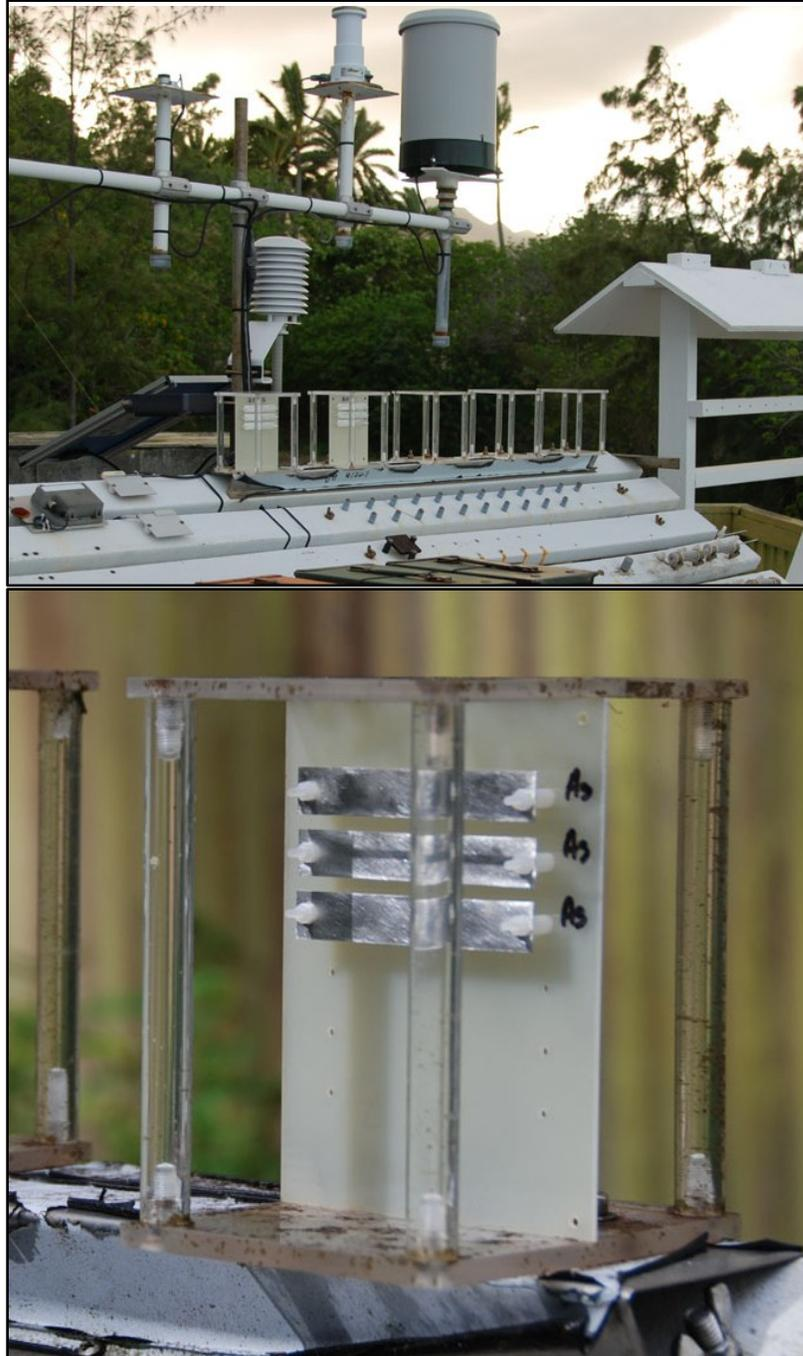
**Figure 2.7** Photographs showing a sample exposure rack typical of those used for the nationwide single-point measurements. The set-up has a slight overhang to minimize contamination and wash-off.
