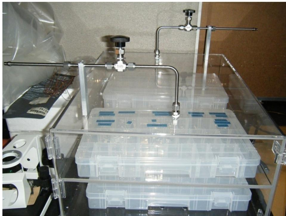
**Figure 2.9** Photograph of the containment box for storing silver samples before/after XPS analysis.
