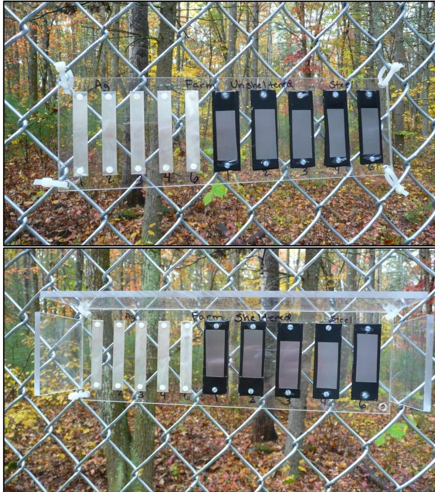
**Figure 2.3** Pictures showing the sample exposures at Thompson Farm, NH. Top is unsheltered and bottom has a slight overhang to minimize contamination and wash-off.
