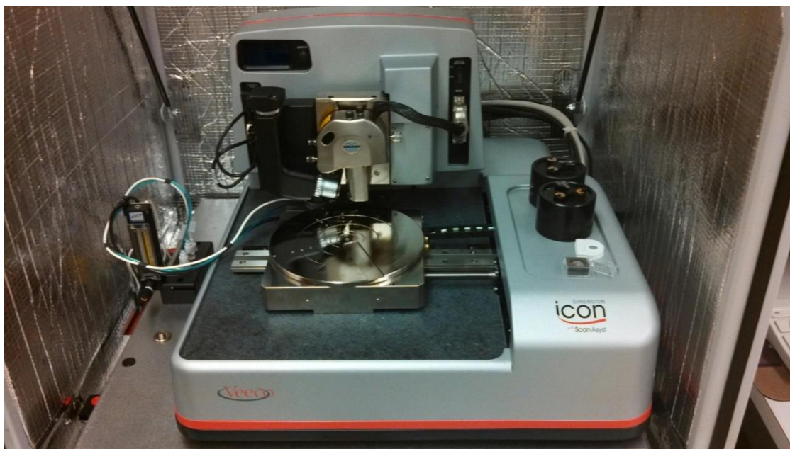
Figure 3.3 The atomic force microscope used for this study at the Surface Analysis Laboratory of the Department of Chemistry and Biochemistry at The Ohio State University.
