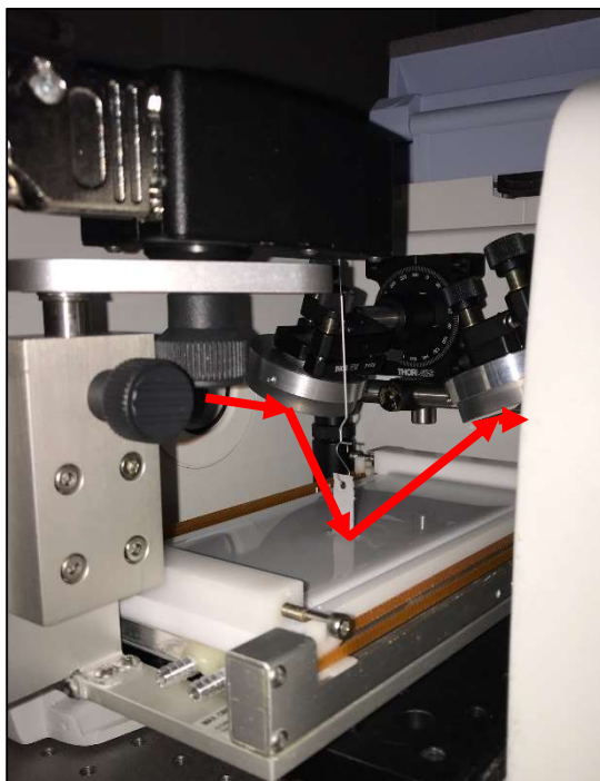
Figure 8: The IRRAS setup housed in the PerkinElmer FTIR spectrometer with a Langmuir trough under the gold mirrors, with the IR beam path shown with red arrows.
