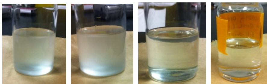
Figure D.1. DPPA (Avanti Polar Lipids) solutions in various solvents. From left to right: 0.0068 g DPPA in 9:1 Ch:Me; 0.0066 g DPPA in 4:1 Ch:Et; 0.0053 g DPPA in 4:1 Ch:Me; 0.0029 g DPPA in 1:1 Ch:Me.
