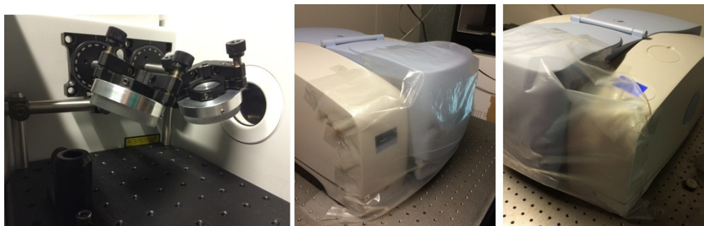
Figure B.3. IRRAS setup used in D_2O experiments. Plastic seals are necessary to prevent atmospheric H_2O condensation onto the aqueous surface.
