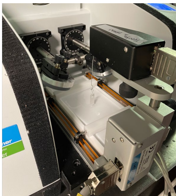
Figure 33. Experimental setup featuring Langmuir trough, barriers, Wilhelmy plate, FTIR spectrometer, and mirrors
