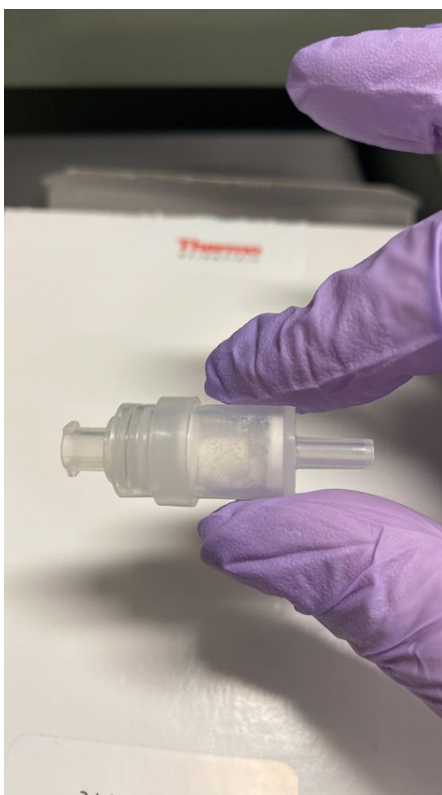
Figure 63. Dionex OnGard II M Cartridges (Product No. 088356, ThermoScientific) for the removal of trace heavy metals in solutions
