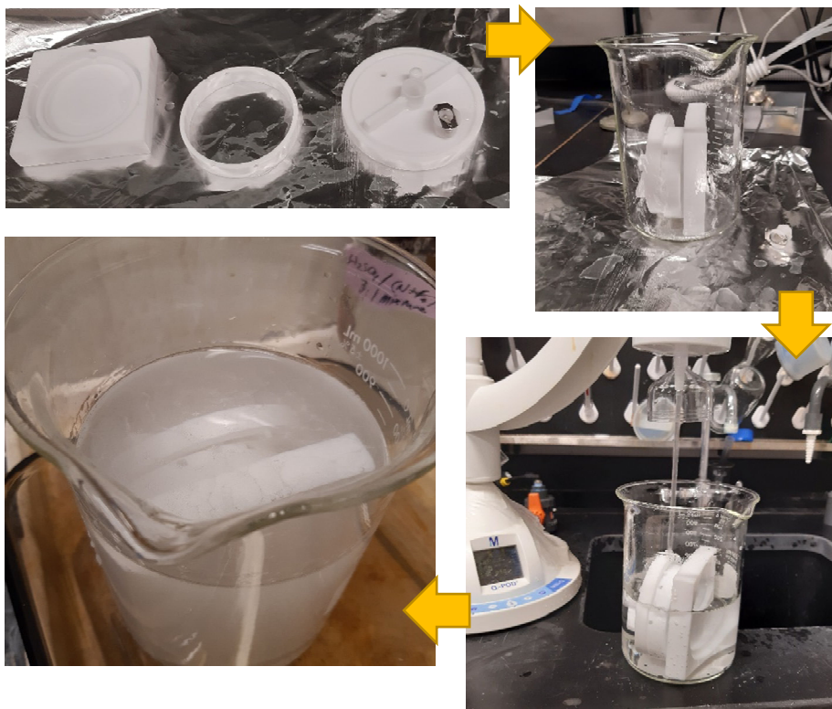
Figure G-1. Sequence of ionizing cell being prepared by rinsing with ultrapure water and being placed in a large acid-cleaned beaker (1000 mL). The inlet for the gas must be unscrewed prior to placement in the beaker. The ionizing cell is soaked in a piranha solution (3:1 sulfuric acid with hydrogen peroxide) for nearly 10-20 mins before quenching in ultrapure water for over 30 mins. The cell is quenched for a total of two 30 min intervals with fresh ultrapure water. The third and final quenching period with fresh ultrapure water is overnight. This process only needs to be done once every couple of weeks before start of a sequence of experiments.
