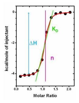
In the case of this simple 1:1 binding experiment, the enthalpy is directly measured/fitted as the heat of 100% binding. The stoichiometry is intuitively denoted by the midpoint of the titration, between 100% binding and 0% binding. The steepness of the rise to saturation is related to binding affinity. For any given system, the steepness of this region is also directly related to the sample concentration.
