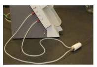
3 Connect the waste line to port **C5** on the left side of the washing module.
