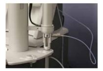
Insert the cell cleaning module into the sample cell. Be sure to push down until the module is firmly seated.
