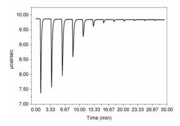
Notice that the first injection results in a larger deflection from the baseline, denoting a larger heat and nearly 100% binding. At the conclusion of the experiment, very little of the injected substance binds, resulting in little or no deflection from baseline (heat).
