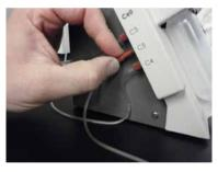
Connect Syringe Needle Cleaning Tube (ASY020512) from the port on the Wash Dry Station on the right side of cell unit (left image below) to port **C2** on the right side of the washing module (right image below).
