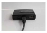
Connect the **USB type A** end of that cable to the labeled **Controller PC USB port**.
