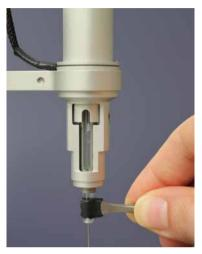
The tip of the tip puller uses a traction design that grabs the plunger tip and allows movement only in one direction.
