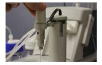
2 Move the pipette and firmly seat into the wash and dry station.
