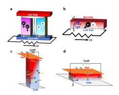
Conventional thermoelectric devices are constructed from two materials arranged in a longitudinal series with one material conducting negatively charged carriers and the other conducting positively charged carriers. Because heat and current flow occur in the same direction, this geometry results in irreversible efficiency losses and thermal degradation of the hot end contacts.
