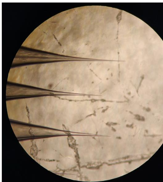
**Fig. 1** Fourfold magnification of the tips of emitters. Nano electrospray emitters with a tip shape as shown generally work well at the spray voltages specified in Table 1.
