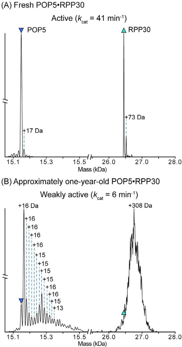
**Fig. 4** Deconvolved zero-charge mass spectra after quadrupole isolation and HCD dissociation of a (POP5-RPP30)<sub>2</sub> charge state. The same preparation of POP5-RPP30 was analyzed and dissociated within (A) 1 month and (B) approximately 1 year after over-expression and purification. Purified POP5-RPP30 is stored at  $-20^{\circ}\text{C}$  as described in *(Continued)*
